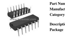
Part NumberM74HCT125B1RManufacturerSTMicroelectronicsCategoryIntegrated Circuits (ICs)<br/>Logic - Buffers, Drivers, Receivers, TransceiversDescriptionIC BUS BUFFER QUAD N-INV 14DIPPackage14-DIP (0.300", 7.62mm)<br/>For the pricing/inventory/lead time, please contact<br/>us<br/>Website: https://www.heisener.com<br/>E-mail: salesdept@heisener.com
