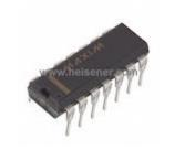
Part NumberMAX491EPD+ManufacturerMaxim IntegratedCategoryIntegrated Circuits (ICs)<br/>Interface - Drivers, Receivers, TransceiversDescriptionIC TXRX RS485/RS422 14-DIPPackage14-DIP (0.300", 7.62mm)<br/>For the pricing/inventory/lead time, please contact<br/>us<br/>Website: https://www.heisener.com<br/>E-mail: salesdept@heisener.com
