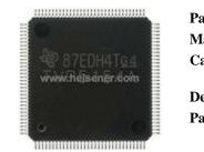
Part NumberTVP5157PNPRManufacturerTexas InstrumentsCategoryIntegrated Circuits (ICs)<br/>Interface - Encoders, Decoders, ConvertersDescriptionIC DECOD VIDEO PAL/NTSC 128HTQFPPackage128-TQFP Exposed Pad<br/>For the pricing/inventory/lead time, please contact<br/>us<br/>Website: https://www.heisener.com<br/>E-mail: salesdept@heisener.com
